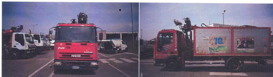
**TELAIO: IVECO 100E21N - ATTREZZATURA: GRU RETROCABINA MEC
